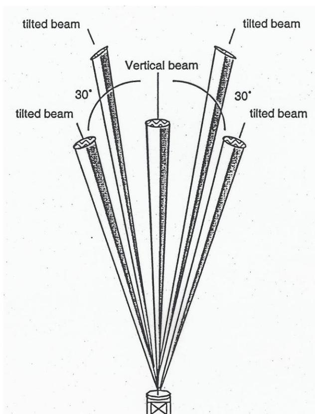
In order to speed up the measurements, in each vertical plane the emission takes place along one tilted beam and its symmetrical beam in sequence and the received signals are processed simultaneously.
